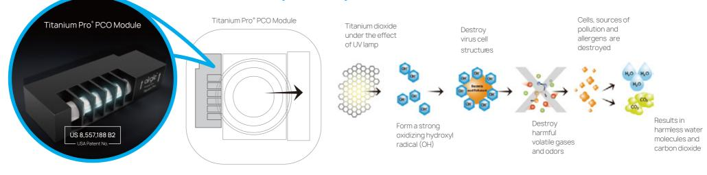
1) The Titanium Pro<sup>®</sup> module creates hydroxyl radicals by exposing titanium oxide (TiO<sub>2</sub>) to ultraviolet light. Hydroxyl radicals are naturally occurring molecules in the atmosphere. In fact, they are often referred to as the "detergent of the troposphere" because hydroxyl radicals destroy many airborne pollutants by breaking apart the molecules of the pollutant.
