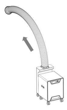
3. To replace the filter and snout, simply pull the snout away from the evacuation arm. Replacement after each use is recommended.
