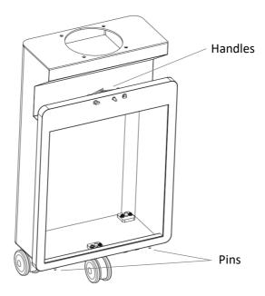
4. Fit the pins at the bottom of the AG900D into corresponding latch holes in the main body of the AG900, as illustrated below.
