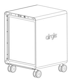
3. Remove the main Housing of the AG900D from the packing box. Make sure the handles air turned toward each other.
