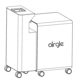
6. Secure the two units together by turning the two handles to the sides to lock the housing into the unit, as illustrated below.
