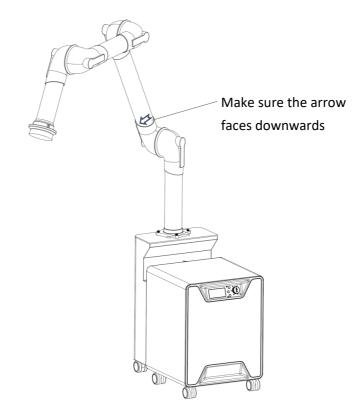
9. Install the disposable filter first and then the suction snout.
