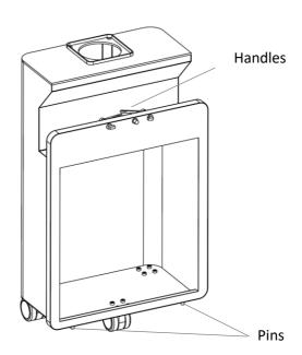
4. Fit the pins at the bottom of the AG600D into corresponding latch holes in the main body of the AG600, as illustrated below.
