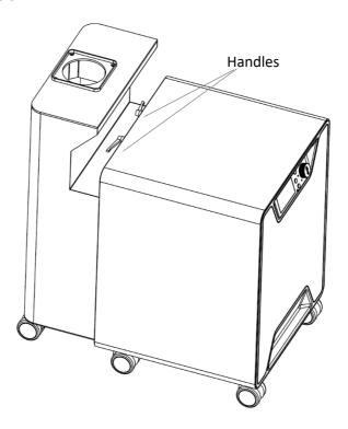
7. Install the AG600D evacuation arm onto the housing.
